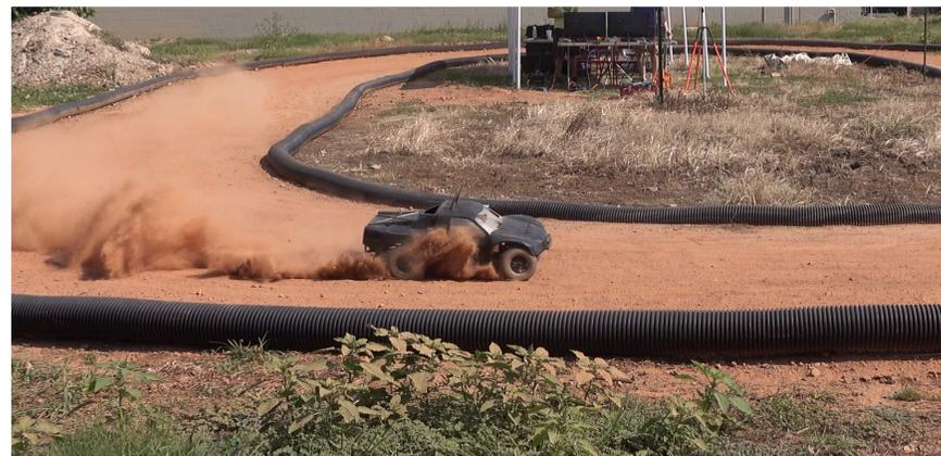
Figure 3 : AutoRally platform power sliding around a corner with the MPPI controller.
