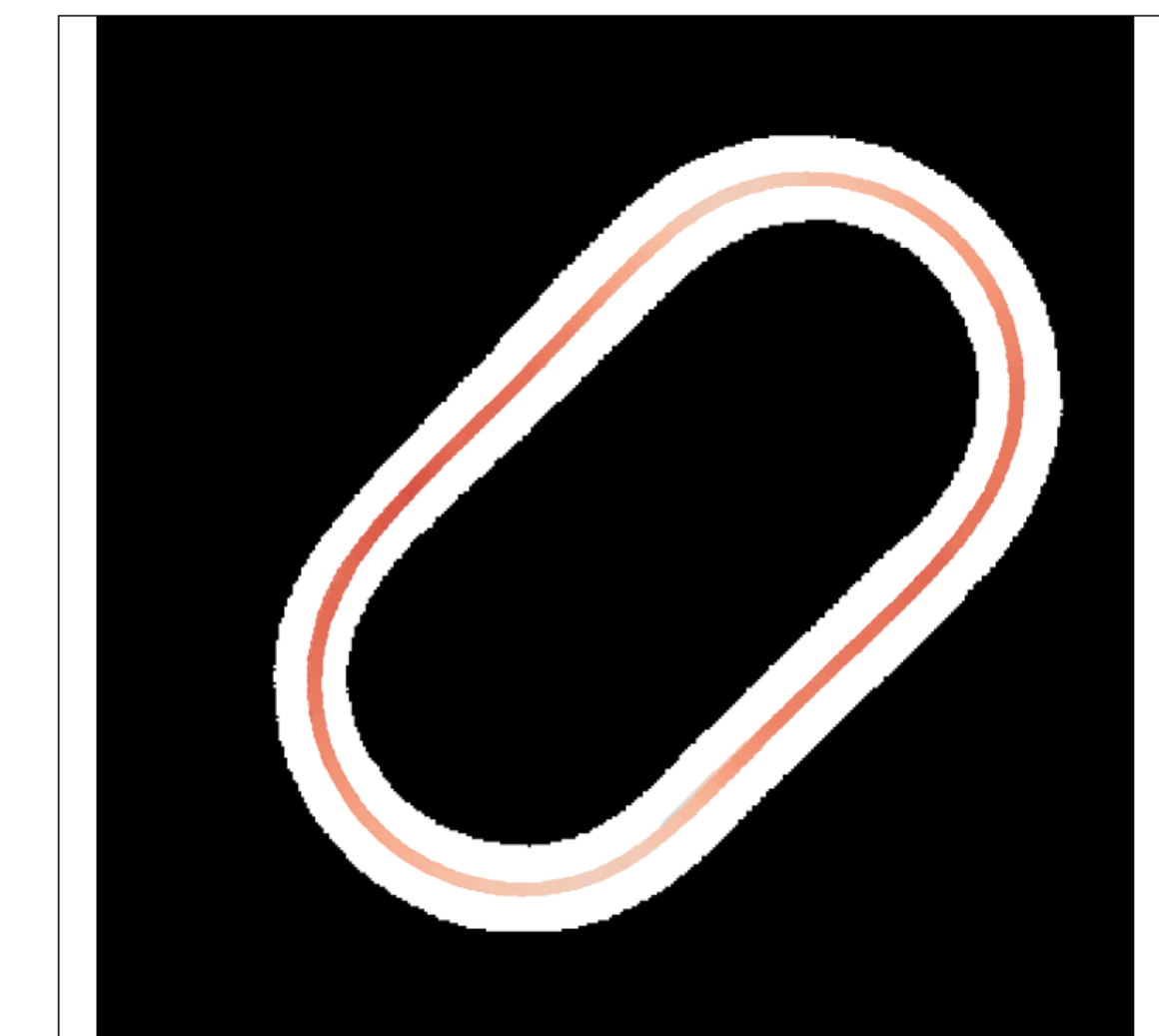
Planning horizon = 1 second Value function used Lap time: 6.50 \pm 0.22 s 0 crashes in 5 trials
